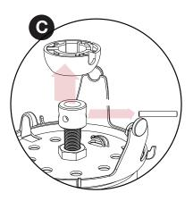
Remove suspension Bolt and Suspension Ball from Motor Shaft
